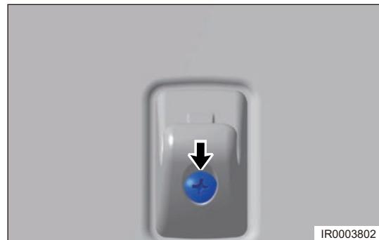
b. Using a screwdriver wrapped with protective tape, pry off the left sun visor holder B (1).
