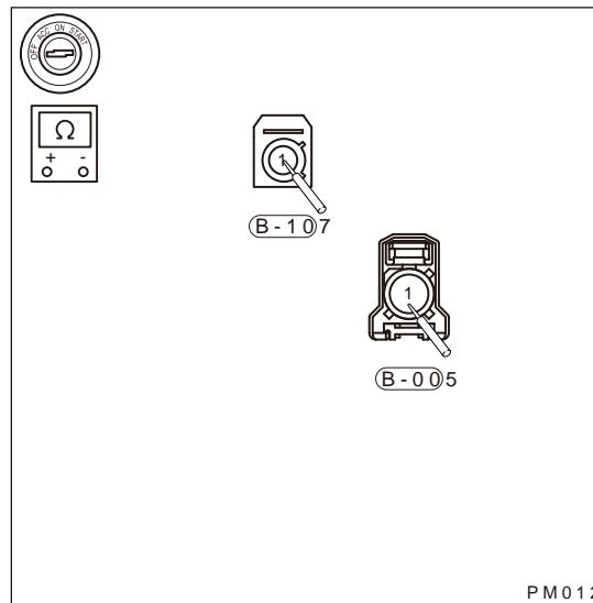
(d) Using ohm band of multimeter, check for continuity between B-107 (D2) and B-005 (2).
