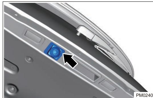
5. Disconnect rear camera connector, pry up fixing clip (1) from camera connector and remove rear camera.
