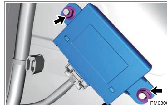
6. Remove the reversing radar control module assembly
