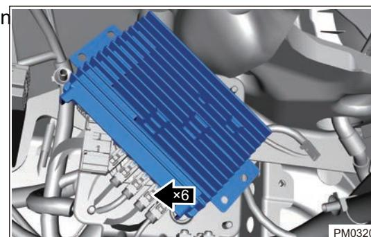
5. Remove 3 fixing bolts from panoramic control system module bracket.
