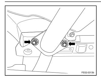
3. Remove the front and rear muffler to the rear muffler retaining nuts and the exhaust pipe gasket.
