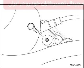
8. Install the three-way catalytic converter right connecting bolt.
