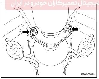
7. Remove the three-way catalytic exhaust converter connecting nuts, remove the exhaust pipe gaskets, remove the three-way catalytic converter and remove the exhaust outlet washers.
