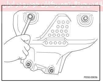
5. Install the exhaust manifold upper heat shield.
