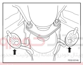
4. Remove the rubber bearings from the front muffler.
