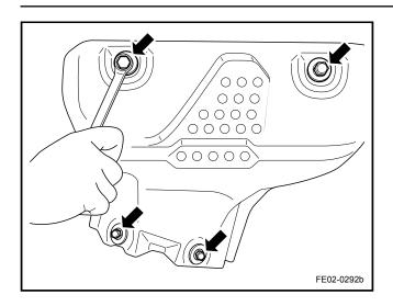
4. Remove heat shield to the exhaust manifold retaining bolts.
