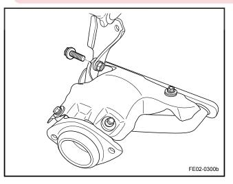
2. Install the exhaust pipe to engine bracket bolts.
