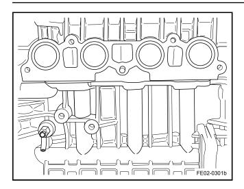
Clean the cylinder head cover and the exhaust manifold mating face.
