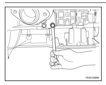
8. Remove the exhaust manifold and exhaust manifold gasket.
