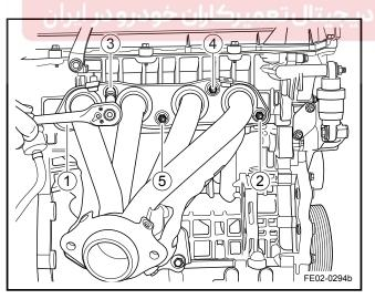
Remove the exhaust manifold bolts and nuts according to the sequence in the graphic.
