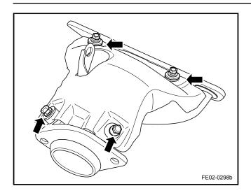
10. Remove the exhaust manifold lower heat shield retaining bolts.
