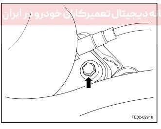
3. Remove the three-way catalytic converter right connecting bolt.
