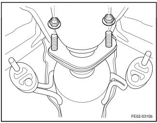
3. Install the exhaust pipe gasket.
