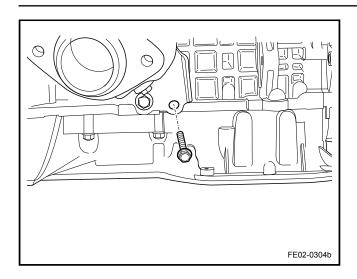
6. Install and tighten the exhaust manifold bracket retaining bolts.
