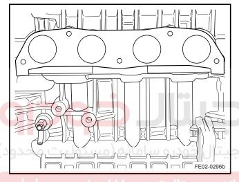
9. Remove the exhaust manifold bracket bolts.
