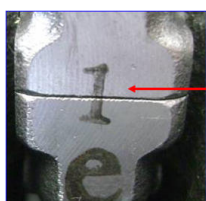
Size grouping code of connecting rod larger end inner diameter
