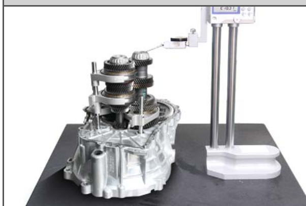
Measuring output shaft height
