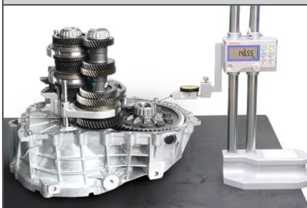
Measuring differential carrier assembly height
