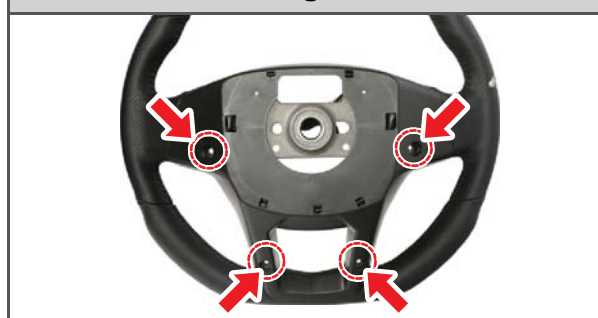
Steering wheel upper cover mounting screws
