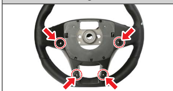
Steering wheel upper cover mounting screws
