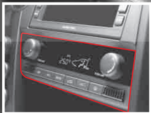
Heater/AC Control Panel
