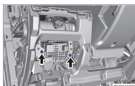
(e) Disconnect the body control module connectors (arrow).
