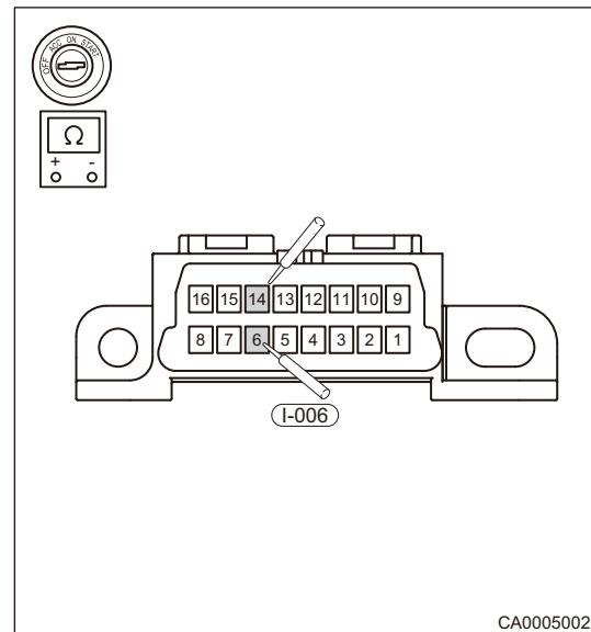
T18 measured value (for reference only): the measured resistance between diagnostic interfaces 6 # and 14 # is  $58.7\ \Omega$  (the two termination resistors are connected in parallel), after the gateway module is disconnected separately, and the measured resistance between diagnostic interfaces 6 # and 14 # is  $\infty$ .
