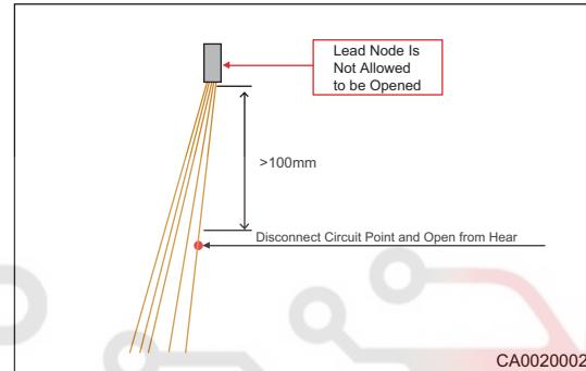
(2) If the CAN line is to be disconnected, it is only allowed to be carried out at a distance of  $\geq 100$  mm from the next pressure node; The twisting of CAN lines is of decisive significance to the interference effect of CAN. Only if the twisting is not damaged, the CAN can be protected from interference, so keep as little interference with the twisting as possible during maintenance.
