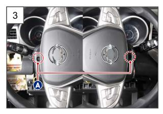
3. Unscrew the 2 shroud lower cover mounting screws (A) by turning the steering wheel.
