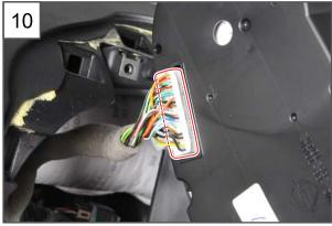
10.Disconnect the connector at the rear side of the instrument cluster.
