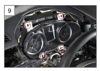
9. Unscrew the 4 mounting screws on the instrument cluster.
