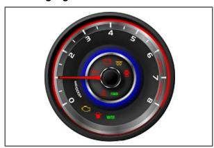
The rpm gauge indicates engine speed in revolutions per minute. Multiply 1,000 to the current number, then it will be the current number of engine revolutions. The ECU receives signal from the crankshaft position sensor and sends it to the instrument cluster via CAN communication. The instrument cluster controls the step motor according to these signals.
