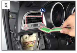
6. Remove the side fascia LH panel from the fixing clips (A) using a hand remover.
