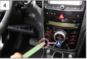
4. Remove the center fascia LH panel by prying off the bottom (A) using a hand remover.
