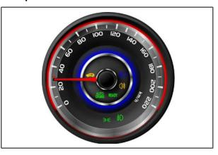
The speedometer indicates the vehicle speed. The ESP sends the wheel speed detected by the 4 wheel speed sensors to the instrument cluster via CAN communication. The instrument cluster calculates autonomously the number of valid signals of the wheel speed signals from the ESP to control the step motor.
