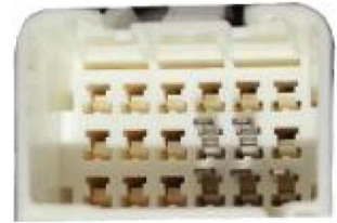
Right front door wire harness
