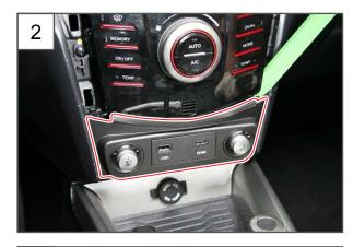
2. Prise apart the center fascia front seat heater switch assembly panel with a hand remover.
