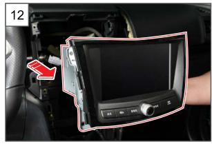
12. Remove the LCD audio head unit.
