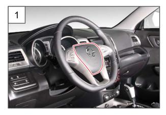
1. Remove the driver air bag module from the steering wheel by following the procedures below:
