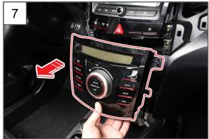
Remove the heater and A/C control assembly.
