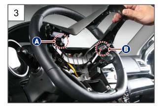
3. Remove the steering wheel upper cover and disconnect the connectors (A) and (B).
