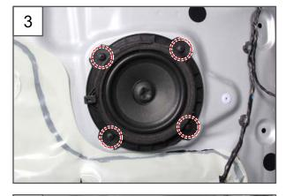
3. Unscrew the 4 mounting screws on the front door speaker.
