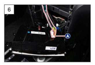
Disconnect the heater and A/C control assembly connector (A) at the rear side of the heat and A/C control assembly by prising the assembly off.
