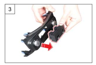
3. Remove the USB and HDMI jack assembly.
