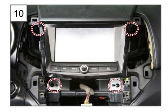
10.Unscrew the 4 mounting screws for the LCD audio head unit and pull it down.
