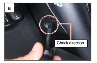
a. Insert a flat bladed screw driver to the 3 holes on the rear side of the steering wheel to press out the snap rings securing the air bag module.
