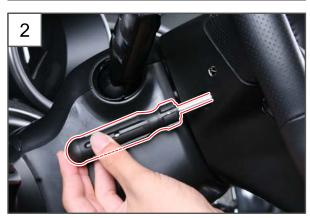
2. Remove the 4 mounting screws for steering wheel upper cover at the back side of the steering wheel.
