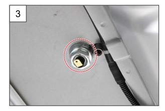
3. Unscrew the mounting nut (19 mm) for the micro pole antenna.
