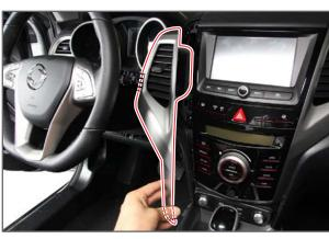
1. Remove the center fascia LH panel by prying off the bottom (A) using a hand remover. (The same method applies to the RH panel.)
