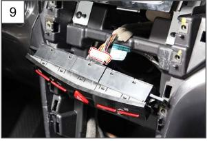
9. Disengage the center fascia switch assembly and pull it down.
