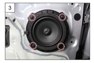
3. Unscrew the 4 mounting screws on the rear door speaker.
