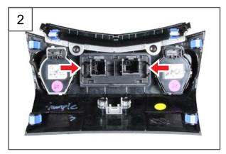
Remove the front seat heater switch assembly.
