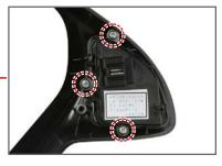
6. Remove the audio remote control switch.
