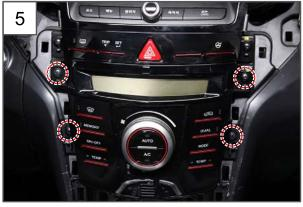
5. Unscrew the 4 mounting screws for the heater and A/C control assembly.
