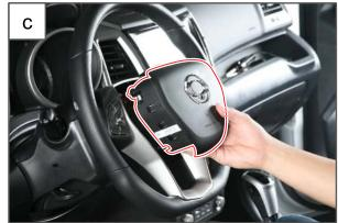
c. Remove the driver's air bag module.
