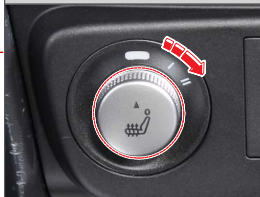
Driver seat heating switch (vehicle with heated wire function only)
