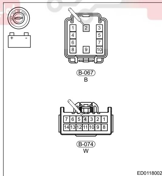
(d) Using ohm band of multimeter, check for continuity between B-074 (104) - B-067 (2), B-074 (11) - B-067 (9) and check if there is open.
