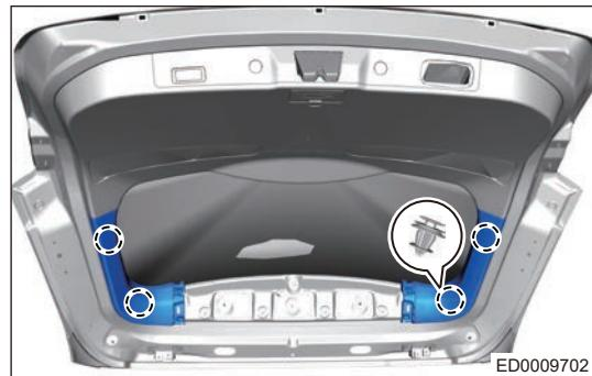
6. Remove the back door mechanical opener trim cover.
