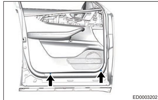
e. Using an interior crow plate, carefully pry off clips on front door inner protector assembly, and loosen front door inner protector assembly in direction of arrow as shown in illustration.
