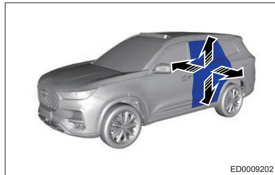
e. Standard ranges of clearance between installation position of rear door assembly and each part are as shown in illustration.
