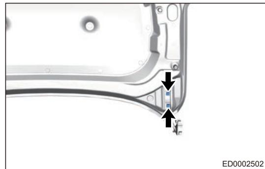
c. Remove 2 fixing bolts (arrow) between engine hood left hinge assembly and body.
