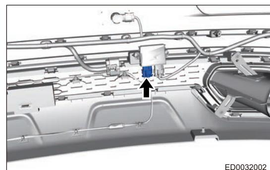
b. Using tools, carefully pry up upper induction antenna fixing clips (1) and remove lower induction antenna (2) to secure 3M sealant (use 3M sealant to secure lower induction antenna).
