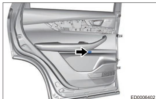
c. Remove 1 fixing screw (arrow) on the rear side of rear door grip lower block cover.
