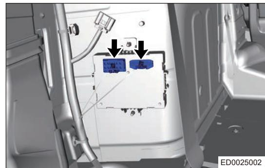
c. Remove the power back door module.
