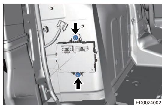
b. Disconnect the power back door module wire harness connectors (arrow).
