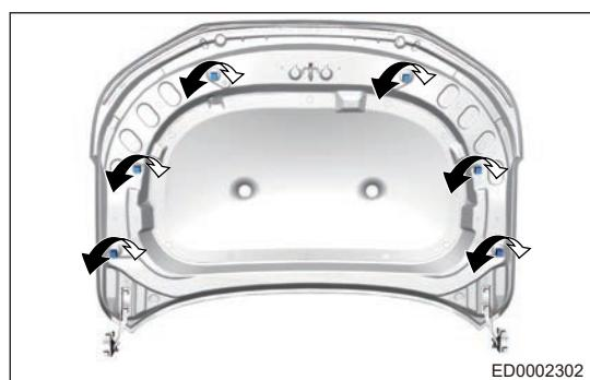
b. After adjustment, make sure that alignment between engine hood assembly and wing assembly is within the standard range.
