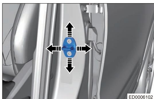
b. Tighten fixing bolts on front door lock striker to specified torque after adjustment.
