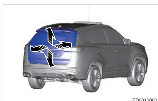
e. Standard ranges of clearance between installation position of back door assembly and each part are as shown in illustration.
