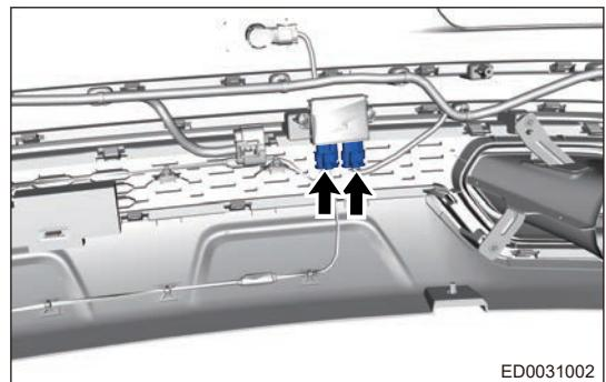
c. Remove the kick sensor module assembly.
