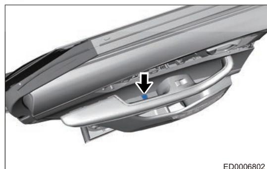
g. Remove 1 fixing screw (arrow) on the rear side of rear door handle box block cover.
