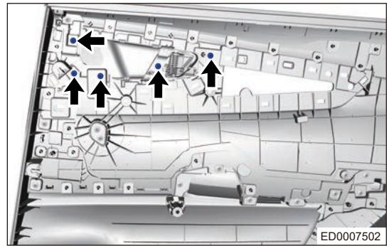
b. Using interior crow plate, pry off claws from rear door inside handle, and remove rear door inside handle.
