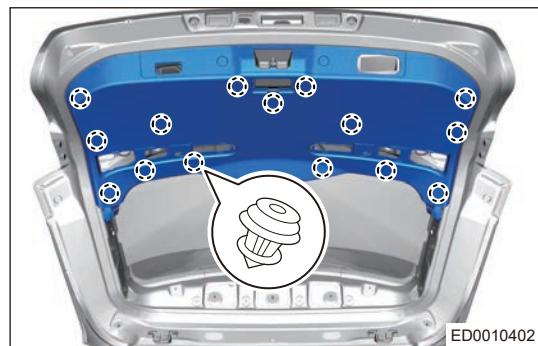
e. Remove the back door lower protector assembly.
