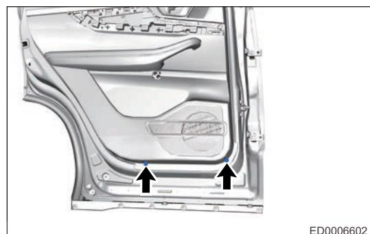
e. Remove the inside handle box cover gasket (arrow).
