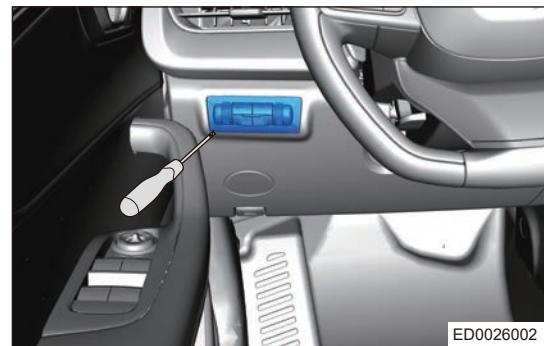
b. Disconnect the power back door instrument cluster switch connector (arrow).
