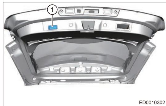
d. Using a screwdriver wrapped with protective tape, pry off claws from back door lower protector assembly.
