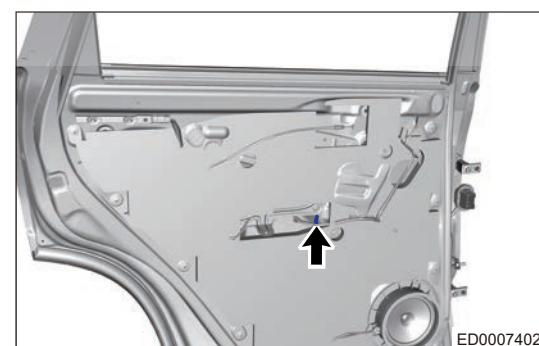
l. Remove the rear left door inner protector assembly.
