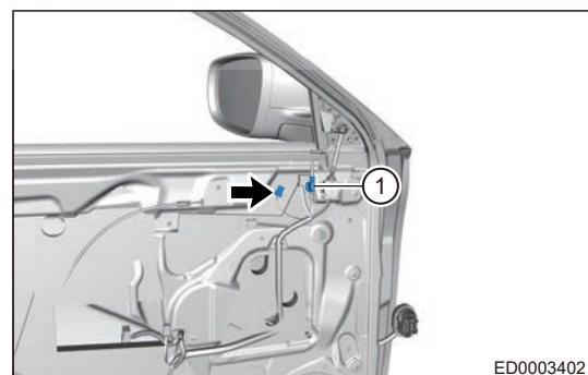
h. Disconnect front door power glass regulator switch connector (arrow) and rear view mirror adjustment switch connector (1).
