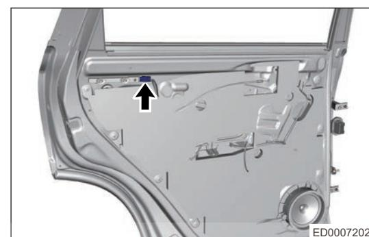
j. Disengage handle cable (arrow) from rear door inside handle.
