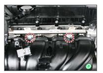
8. Remove the fuel rail assembly from the intake manifold by grasping and pulling it with both hands as shown in the picture.
