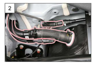
2. Disconnect the 3 fuel filler assembly hoses from the fuel tank located under the vehicle.
