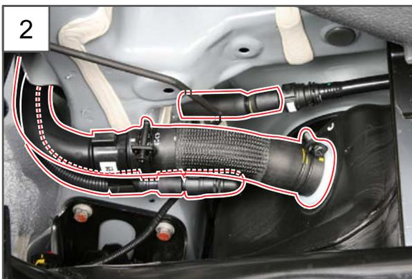
2. Disconnect the 3 fuel filler assembly hoses from the fuel tank located under the vehicle.
