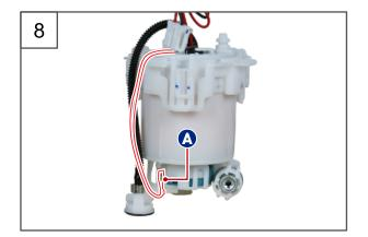
8. Remove the ground wire (A) and assist valve (B) from the fuel filter assembly.
