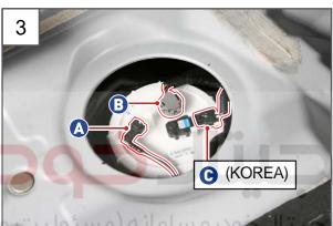
2. Remove the fuel pump dust cover using a hand remover.
