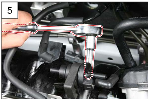
5. Unscrew the PCSV mounting bolt (10 mm).
