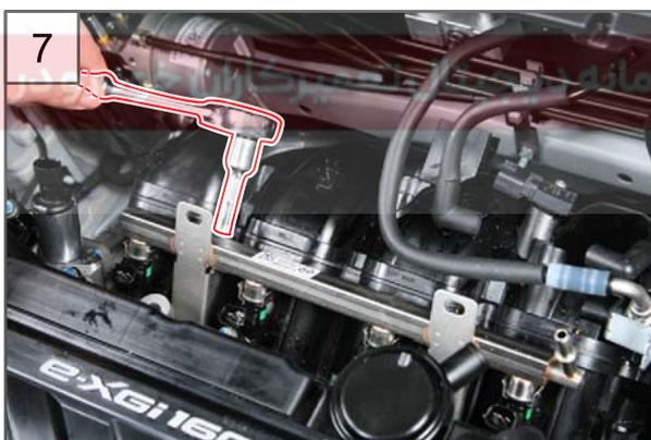
7. Unscrew the 2 mounting bolts (13 mm) securing the fuel rail assembly on the top of the intake manifold.
