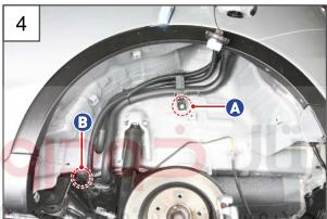
4. Unscrew the middle mounting nut (A, 10 mm) and lower mounting bolt (B, 10 mm) for the fuel filler assembly.
