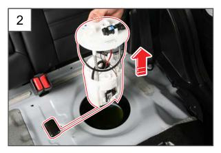
2. Remove the fuel pump assembly from the vehicle.
