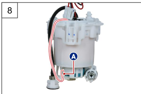
8. Remove the ground wire (A) and assist valve (B) from the fuel filter assembly.
