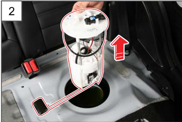
2. Remove the fuel pump assembly from the vehicle.
