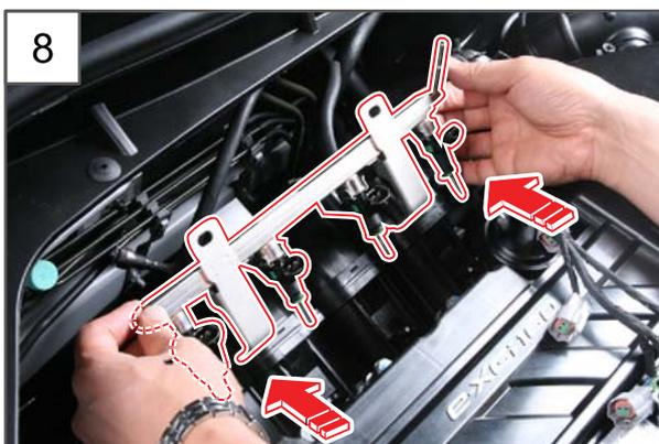
8. Remove the fuel rail assembly from the intake manifold by grasping and pulling it with both hands as shown in the picture.
