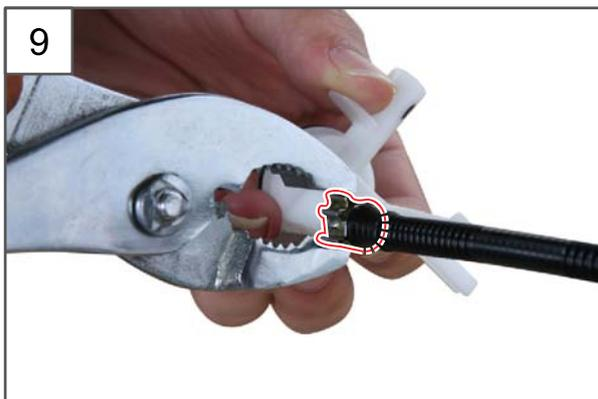
9. Disengage the mounting clip to remove the assist valve.
