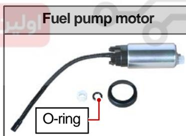
11. Remove the fuel pump motor from the fuel filter assembly.
