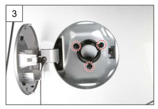
3. Open the fuel filler cap and unscrew the 3 mounting bolts (10 mm) on top of the fuel filler assembly.
