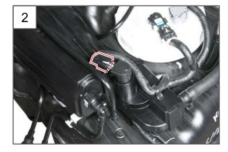
Disconnect the canister shut off valve connector on the top of the air filter of the removed fuel tank assembly. (KOREA)
