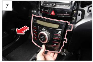
7. Remove the heater and A/C control assembly.
