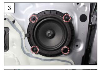
3. Unscrew the 4 mounting screws on the rear door speaker.
