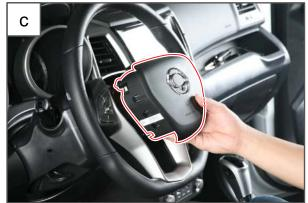
c. Remove the driver's air bag module.
