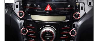
5. Unscrew the 4 mounting screws for the heater and A/C control assembly.
