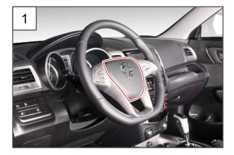
Remove the driver air bag module from the steering wheel by following the procedures below:
