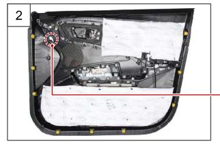
2. Disengage the mounting for the front tweeter speaker.
