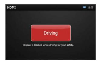
During driving, only the sound of the video file is played. The image of the video file does not appear on the screen. (The image will appear on the screen as soon as the vehicle stops.)
