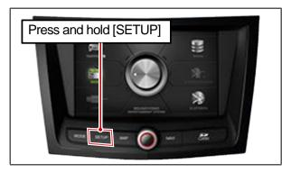
1. Press and hold the [SETUP] hard key under the AVN head unit front screen for 1.5 sec. or more.
