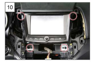
10.Unscrew the 4 mounting screws for the AVN head unit and pull it down.
