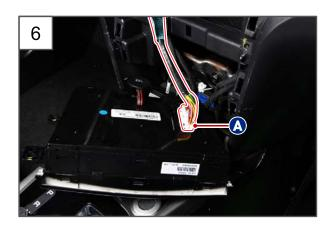
Disconnect the heater and A/C control assembly connector (A) at the rear side of the heat and A/C control assembly by prising the assembly off.
