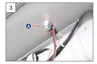
3. Unscrew the mounting nut (19 mm) for the integrated micro pole antenna.
