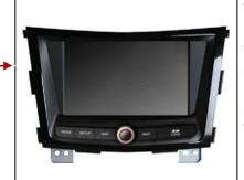
The AVN system plays radio, audio and video files in various formats. The system also has navigation and Bluetooth functions. The system is equipped with the touchscreen for the best user experience.
