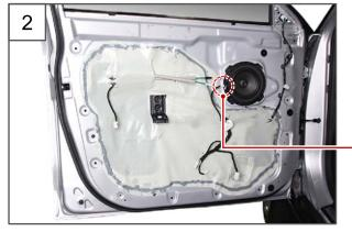
2. Disconnect the front door speaker connector (A).
