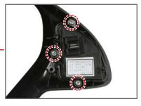
6. Remove the audio remote control switch.
