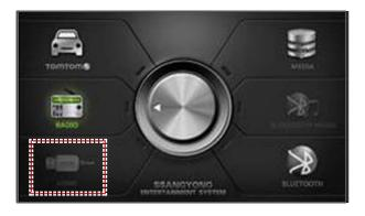
2. Select [HDMI] button to run HDMI mode. If no device is connected to the HDMI jack, the system will not enter HDMI mode.
