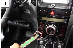
1. Remove the center fascia LH panel by prying off the bottom (A) using a hand remover. (The same method applies to the RH panel.)
