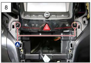
8. Unscrew the 2 mounting screws (A) for the center fascia switch assembly.
