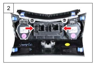
Remove the front seat heater switch assembly.
