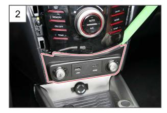
2. Prise apart the center fascia front seat heater switch assembly panel with a hand remover.
