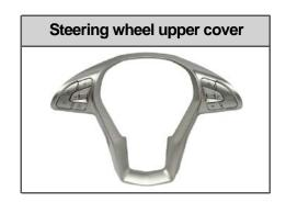
5. Remove the 3 mounting screws for the audio remote control switch at the back side of the steering wheel upper cover.
