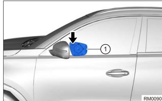
6. Disconnect the connector from rear view mirror lens assembly, and remove the left outside rear view mirror lens assembly (1) (if equipped with rear view mirror heater).
