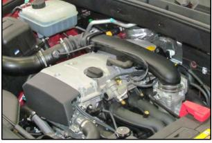
6. Disconnect the coupling of HFM sensor and remove the air cleaner cross pipe.
