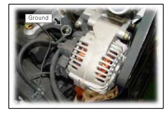
9. Disconnect the parts connected to the engine from the engine compartment.
