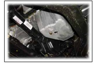
4. Remove the drain plug and drain the engine
