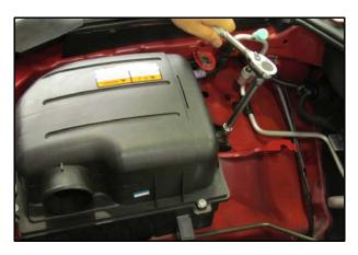
7. Remove the air cleaner cover. Remove the mounting bolts and air cleaner housing and element assembly.
