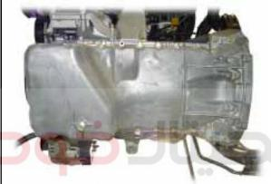
2. Unscrew the bolts and remove the oil pan and gasket.
