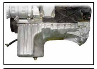
1. Remove the drain plug and drain the oil completely.
