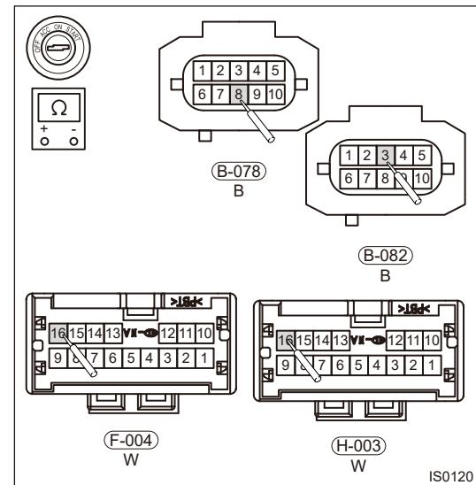
(c) Using ohm band of multimeter, check for continuity between F-004 (9) or H-003 (9) and body ground separately.
