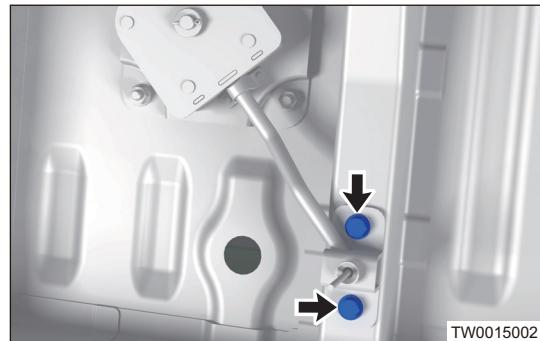
2. Remove 4 nuts (arrow) between spare tire lifter and body.
