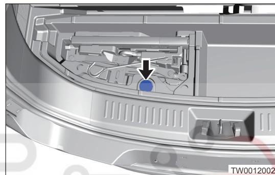
4. Use the extended wrench of tool kit to fit hex head of spare tire lifter (in luggage compartment plastic storage box) and turn hex head counterclockwise until spare tire falls to ground from the bottom of luggage compartment.
