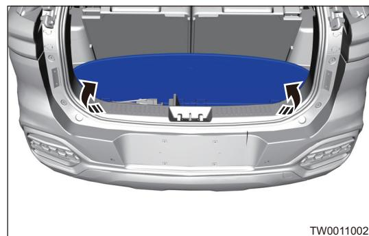
3. Pry off the spare tire lifter plastic cover (arrow) carefully. (In luggage compartment plastic storage box).
