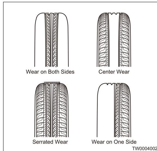
4. Measure the tread pattern depth with a tire depth gauge. When the depth is less than 1.6 mm, the tire should be replaced.
