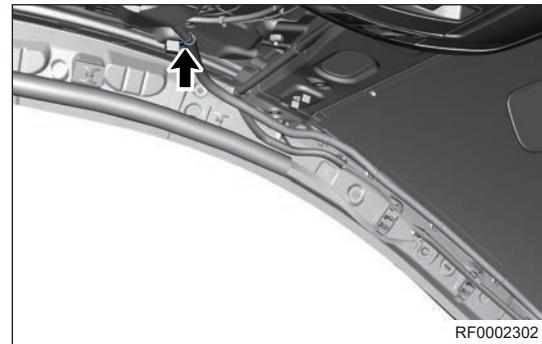
b. Using an interior pry bar, carefully pry off band (arrow) from front left drain hose.
