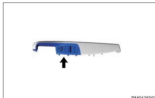
c. Using an interior crow plate, pry off claws (arrow) and remove the outside rear view mirror adjustment switch.
