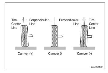
Camber is the tilting of the top of the tire from the vertical when viewed from the front of the vehicle. When the tires tilt outward, the camber is positive. When the tires tilt inward, the camber is negative. The camber angle is measured in degrees from the vertical. Camber influnces both directional control and tire wear.
