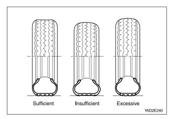
2. Inspect the pressure of the tire surface and check the inflation pressure.
