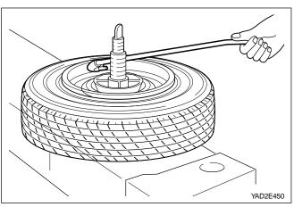
5. Check any foreign material or liquid for the tire inside and then install to push down the tire.
