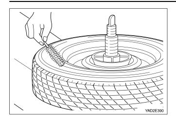
5. Apply the lubricant between the rim and the bead.
