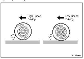
The condition of driving a vehicle fast on the road surface covered with water can cause tires to fail to rotate with a good contact on the surface, so results in remaining them a float. This is so-called hydroplaning. It causes brake failure, lower tractive force and losing the steering performance so it is very vulnerable condition.
