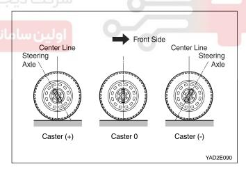
Caster is the tilting of the uppermost point of the steering axis either forward or backward from the vertical when viewed from the side of the vehicle. A backward tilt is positive and a forward tilt negative. Caster influences directional control of the steering but does not affect tire wear.
