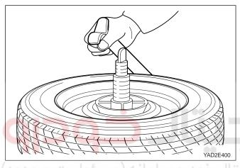
6. Insert the removal lever between the tire's bead and the rim and separate the rim from the tire.
