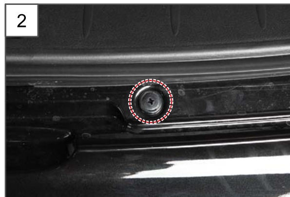
2. Unscrew four rear mounting screw rivets.
