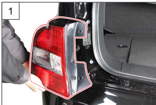
1. Remove the rear tail lamp assembly.
