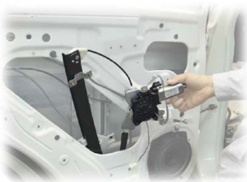
Removal of Window Regulator
