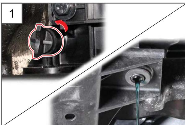
1. Drain the coolant. Refer to "COOLANT DRAIN AND FILL UP" under "REMOVAL AND INSTALLATION" subsection of "COOLING SYSTEM" section in "G16DF ENGINE" chapter.
