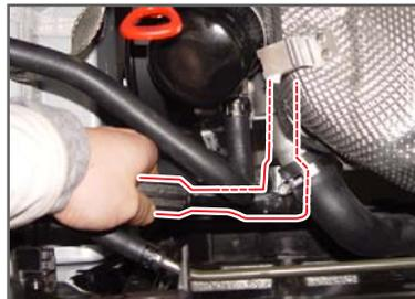
3. Remove the oil pressure switch.
