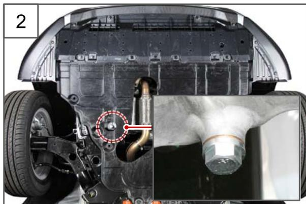
2. Unscrew the oil pan drain plug (14 mm) under the vehicle to drain the engine oil. Fit the drain plug after the oil has been drained completely.
