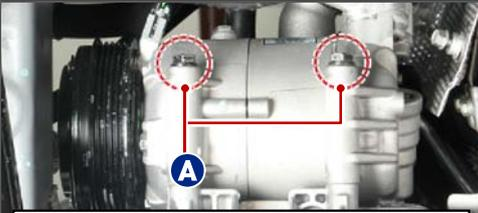
**Tightening torque** 25 ± 2.5 Nm
