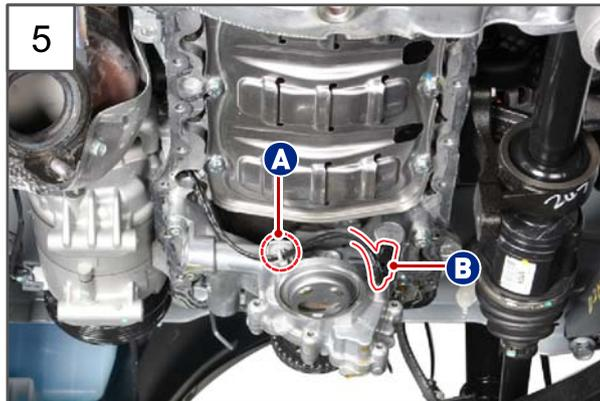
5. Disengage the VOP extension wiring clamp (A) and disconnect the VOP solenoid connector (B) from the oil pump.
