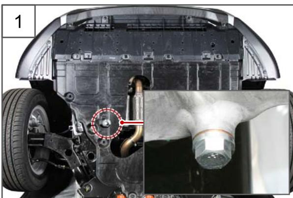
1. Unscrew the oil drain plug (14 mm) under the vehicle to drain the engine oil.
