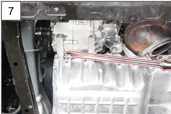
7. Pry off the oil pan by inserting a flat-bladed screwdriver into the gap between the oil pan and A/C compressor.
