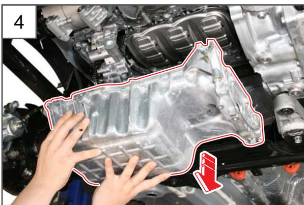
4. Remove the oil pan from the vehicle.
