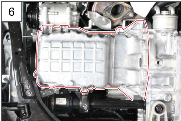
6. Unscrew the mounting bolts (A), (B), (C), and (D) for the oil pan from the underside of the engine assembly.
