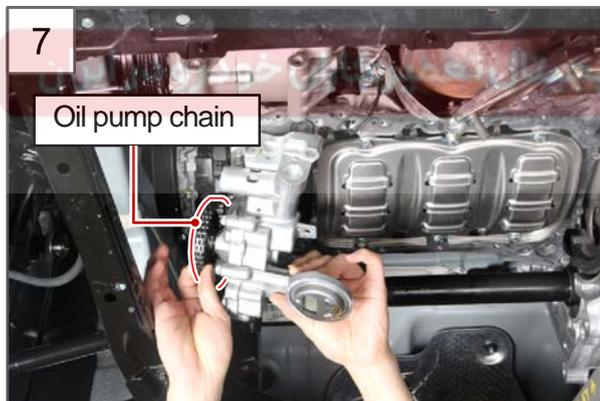
7. Separate the oil pump from the oil pump chain.
