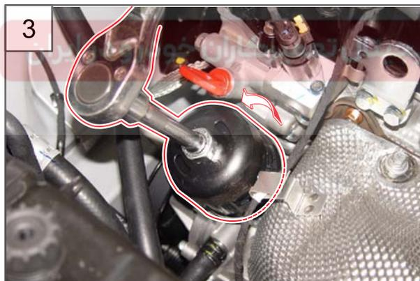
3. Loosen the oil filter in the engine compartment with an oil filter removal/installation cup by turning it counterclockwise.
