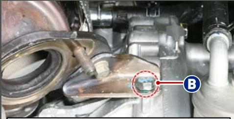
**Tightening torque** 25 ± 2.5 Nm
