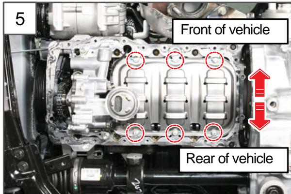
5. Unscrew the 6 mounting bolts (10 mm) for the baffle plate.
