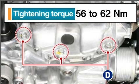
**Tightening torque** 56 to 62 Nm
