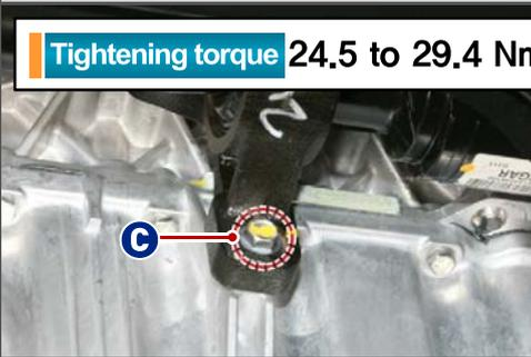
**Tightening torque** 24.5 to 29.4 Nm
