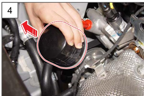
4. Remove the oil filter and replace it with a new one.
