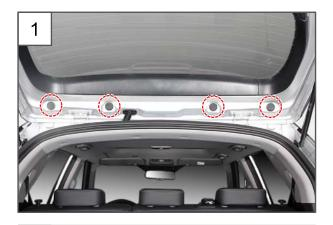
1. Remove the 4 blind plugs after opening the tailgate.
