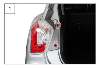
1. Unscrew the 2 mounting screws for the rear combination lamp.
