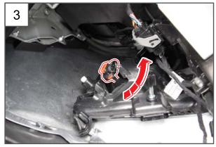
3. Turn the fog lamp bulb in the direction of the arrow to remove it.
