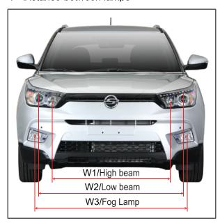
W1: Distance between high beams W2: Distance between low beams W3: Distance between fog lamps H1: Low beam ground clearance H2: High beam ground clearance H3: Fog lamp ground clearance
