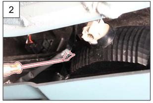
2. Disengage the retaining key for the rear fog lamp wiring with a flat bladed screwdriver.
