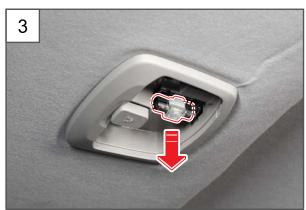
3. Remove the center room lamp bulb.
