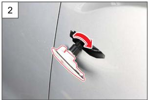
2. Turn the side repeater lamp lens to remove it.
