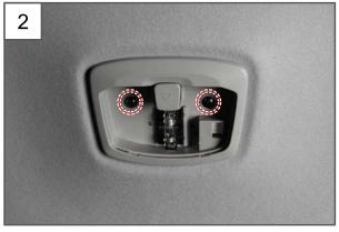
2. Unscrew the 2 mounting screws for the center room lamp.
