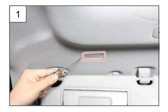
1. Separate the sun visor lamp assembly from the headlining using a flat-bladed screwdriver.
