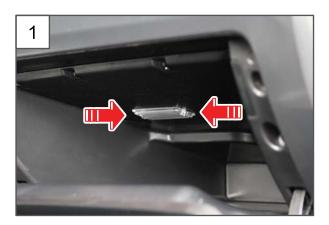
1. Pry off the points indicated by the arrows to pull out the glove box lamp assembly.
