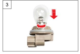
3. Turn the rear fog lamp bulb in the direction of the arrow to remove it.
