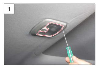
1. Prise apart the center room lamp bulb lens using a flat-bladed screwdriver.
