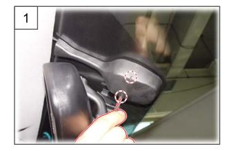
1. Insert a screwdriver into the service holes at both sides of the styling cover to remove the cover.
