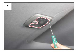
1. Prise apart the center room lamp bulb lens using a flat-bladed screwdriver.
