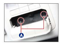
2. Detach the overhead console by disengaging the clips (A).
