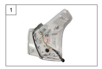
Turn the rear turn signal lamp bulb socket in the direction of the arrow at the rear side of the rear combination lamp assembly to remove it.
