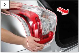
2. Slide the rear combination lamp in the direction of the arrow to remove it.
