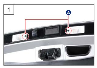
1. Remove the mounting screws (A) for the license plate lamps from the tailgate rear garnish.
