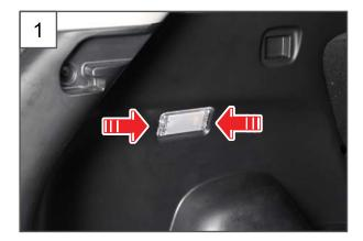
1. Pry off the points indicated by the arrows to pull out the luggage room lamp assembly.
