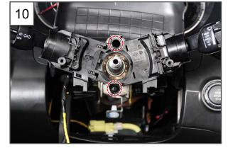
10. Remove the 2 mounting screws for the multifunction switch assembly.
