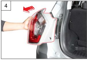
4. Remove the rear combination lamp assembly.
