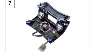
7. Unscrew the 2 mounting screws for the IP center lower mood lamp.
