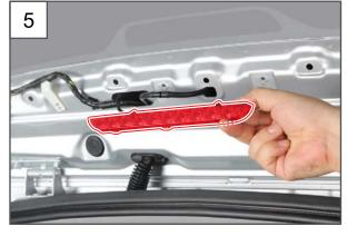
5. Remove the high mounted stop lamp.
