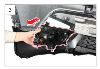
3. Remove the front fog lamp assembly.
