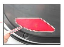
2. Remove the front door courtesy lamp lens.
