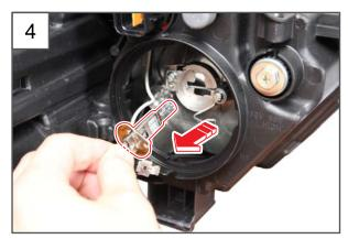
4. Remove the high beam bulb.
