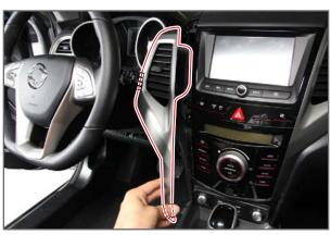
1. Remove the center fascia LH panel by prying off the bottom (A) using a hand remover. (The same method applies to the RH panel.)
