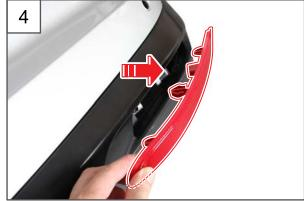
4. Remove the reflex reflector lamp assembly.
