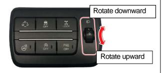
With the headlights ON, the level of headlight can be adjusted in 4 stages (0~3 level) by turning the switch when the vehicle heights of front and back are different due to the number of passengers and the loading conditions of the vehicle.
