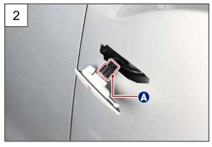
2. Disconnect the side repeater lamp connector (A).
