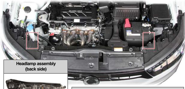
Headlamp leveling device fitted at the back side of headlamp assembly can adjust headlamp aiming angle.
