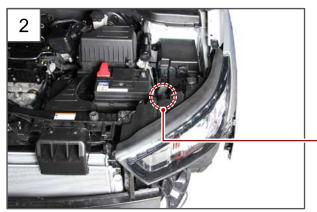
2. Disconnect the headlamp connector (A) on the upper side of the headlamp.
