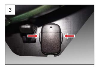
3. Insert a screwdriver into the service holes at both sides of the cover to separate between the upper and lower covers.
