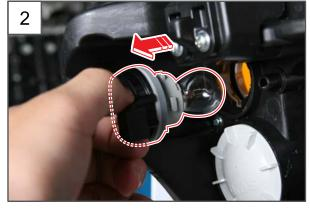
3. Remove the turn signal lamp bulb from the socket while pressing it downward.
