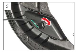
3. Turn the door courtesy lamp assembly in the direction of the arrow to remove it.
