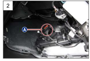
2. Separate the wheel house cover and disconnect the front fog lamp connector (A).
