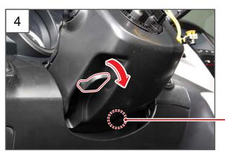
Unscrew the mounting screw (A) for the shroud lower panel, and push down the steering column tilting lever in the direction of the arrow.
