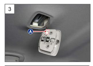
3. Disengage the center room lamp assembly and disconnect the connector (A).
