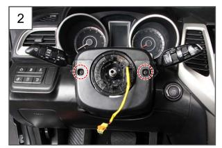
2. Unscrew the 2 mounting screws on the shroud upper and lower panels.
