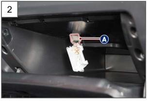
2. Disconnect the glove box lamp assembly connector (A).
