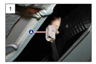
1. Disconnect the rear fog lamp connector (A) at the rear side of the rear bumper.
