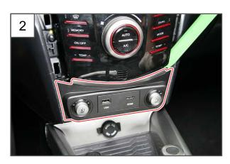
2. Separate the center lower panel using a hand remover.
