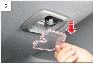
2. Remove the center room lamp bulb lens.
