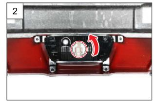
2. Turn the rear fog lamp bulb socket in the direction of the arrow to remove it.
