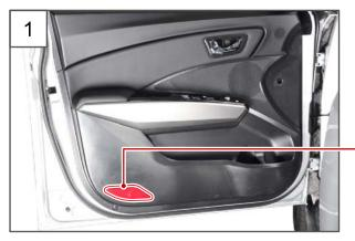
1. Prise apart the front door courtesy lamp lens using a flat-bladed screwdriver.
