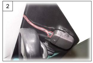
2. Disconnect the connector from the AUTO light and rain sensor module.
