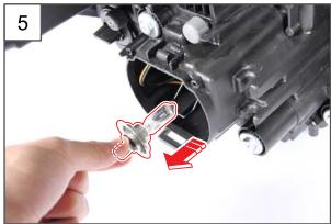
5. Pull out the low beam bulb in the direction of the arrow to remove it.
