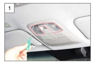
1. Prise apart the front room lamp bulb lens using a flat-bladed screwdriver.
