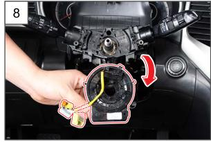
8. Remove the contact coil assembly.
