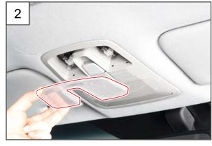
2. Remove the front room lamp bulb lens.
