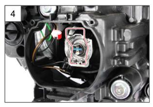
4. Press the low beam bulb retaining pin in the direction of the arrow to detach it.
