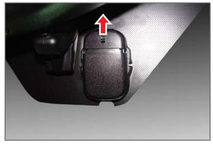
4. Pull out the AUTO light sensor module in the direction of the arrow to remove it.
