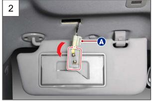
2. Disconnect the sun visor lamp connector (A).
