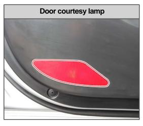
The door courtesy lamp comes on when the driver's door or passenger's door is opened.
