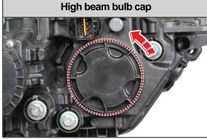
2. Disconnect the connector (A) for the bulb of the high beam.
