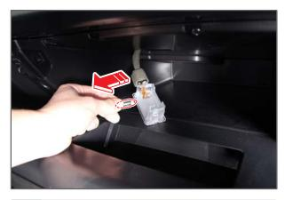
3. Install the new bulb in the reverse order of removal.
