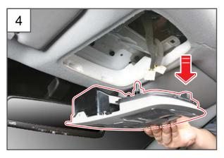
4. Remove the overhead console switch assembly.
