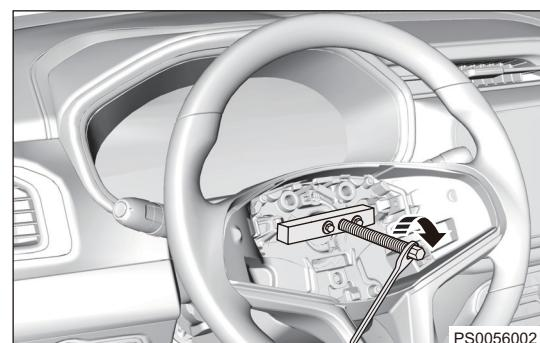
(c) As shown in the illustration, install the steering wheel remover, and then tighten it with a wrench to loosen the steering wheel assembly from steering column assembly.
