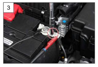
Unscrew the mounting nut (12 mm) to separate the battery ground cable from the negative (-) battery terminal.
