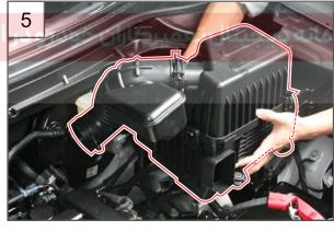
5. Remove the air cleaner housing with the air cleaner hose.
