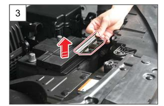
3. Remove the battery clamp.
