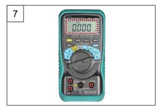
Measure the current when the system enters sleep mode after 3 minutes have passed since the separation of ground cable and battery negative terminal.
