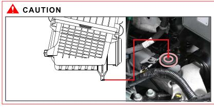
When installing the air cleaner housing, make sure that the retaining key at the bottom of the housing is seated correctly on the recessed area of the engine compartment.
