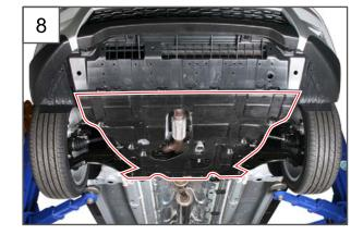
8. Remove the rear under cover under the vehicle.
