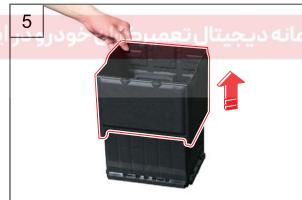
5. Separate the battery cover from the removed battery.
