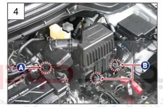
4. Remove the spring clamp (A, 10 mm) for the air cleaner hose and 2 mounting bolts (B, 12 mm) for the air cleaner housing.
