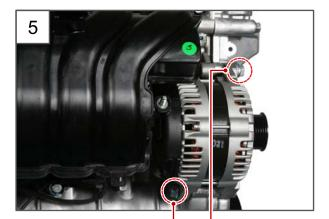
5. Unscrew the mounting bolt (A, 15 mm) and (B, 17 mm) for the alternator.
