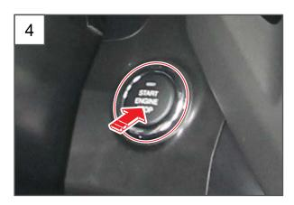
4. Turn the ignition on. Once the voltage has been supplied to the various units turn the ignition off.
