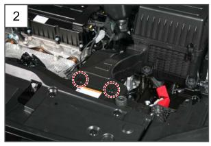
2. Remove the 2 screw rivets securing the snorkel assembly.
