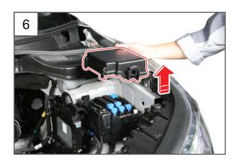
6. Remove the fuse box in the engine compartment.
