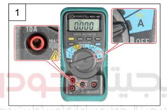
1. Set the current measuring range of the ammeter to 10 A.
