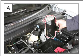
A. Remove the fuel filter assembly.
