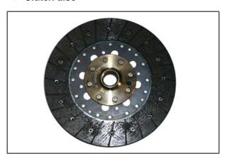
The clutch disc is installed between the engine flywheel and the pressure plate. The spline part is installed in the center of the disc and transmits the engine's electric power to the transmission. The transmission input shaft can be inserted into the spline part. The clutch disc has friction materials on its edges, where the engine power can be interrupted, and the cushion spring is installed to prevent friction materials (facing) from unevenly wearing out.
