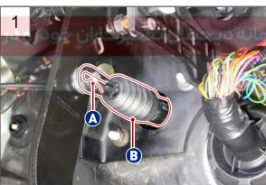
1. Remove the twist pin (A) and remove the clutch master cylinder push rod (B) from the clutch pedal.
