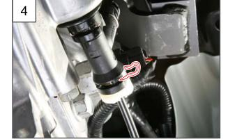
4. Remove the oil tube mounting pin from the air bleeder on the transmission side.
