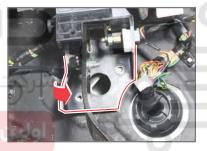
2. Turn the clutch pedal in the direction of the arrow (B) to remove it, taking into account the interference with other parts.
