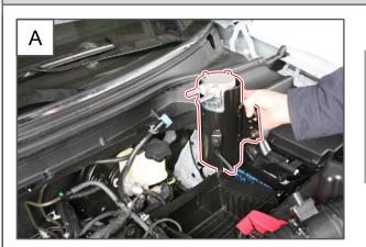
A. Remove the fuel filter assembly.
