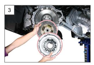
3. Unscrew the mounting bolts completely and remove the clutch cover assembly and clutch disc.
