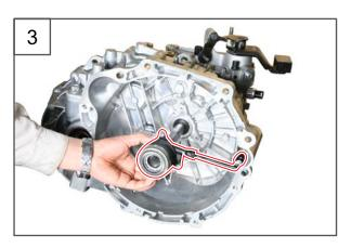
3. Remove the concentric slave cylinder from the transmission input shaft. Also, disconnect the oil pipe connected to the cylinder, at this time.
