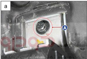
a. Remove the mounting bolt (A, 12 mm) for the clutch pedal.
