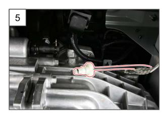
5. Disconnect the oil tube from the air bleeder.
