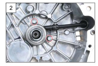
2. Unscrew the 2 mounting bolts (10 mm) for the concentric slave cylinder from the clutch housing of the removed M/T transmission.
