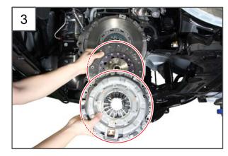
3. Remove the clutch cover and clutch disc.
